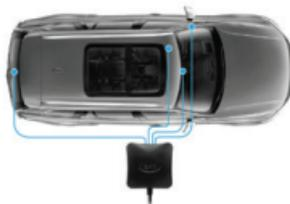
External GPS antenna is attached using a built-in magnet when installed in a rack or on other elements of the car body. In other cases, it is possible to mount the antenna using double-sided 3M tape. Connect the antenna to the Main HUB using the connection cable to the "GPS antenna" port.
