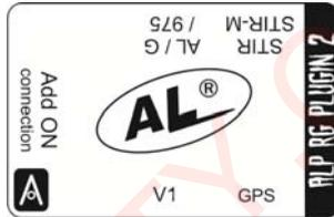
2. Connect the other side of the cable by plugging the connector into the Add-on socket on your AL Priority Control Box.
