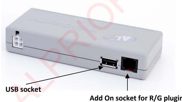
3. Connect your radar antenna to appropriate socket on the ALP R/G plugin.
